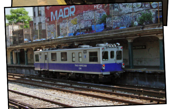
Geometry trains hard at work detecting which sections of the subway need repairs
